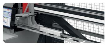
• Conveys the processed profiles to cutting unit.
