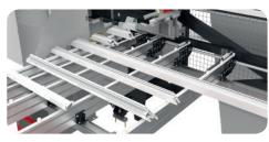
Output robot conveys the cut profiles on conveyor automatically.
