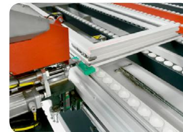
• Fast and accurate screwing of espagnolette with screwing unit.
